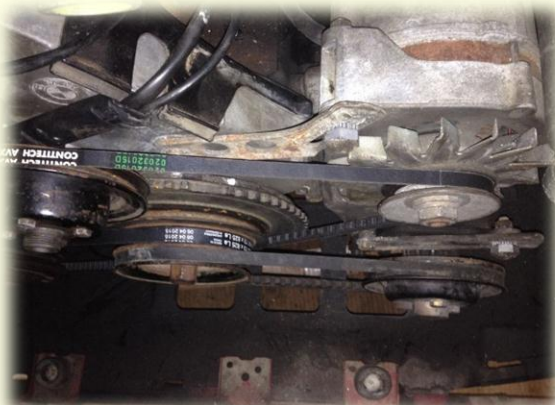
Fan belt running alternator and water pump (top), power steering belt (right), and a/c compressor belt (left, bottom) on a 1987 BMW E30 325is
